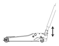
7. Jack is now ready for use. Check for proper pump action. (Repeat steps if necessary).
