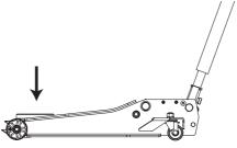
▲ WARNING: WARNING: USE EXTREME CAUTION WHEN LOWERING THE JACK. THE JACK HANDLE MAY TURN RAPIDLY. OPENING THE RELEASE VALVE TOO FAST CAN CAUSE THE JACK TO LOWER RAPIDLY. FAILURE TO HEAD THESE WARNINGS COULD CAUSE SERIOUS INJURY OR DEATH.
