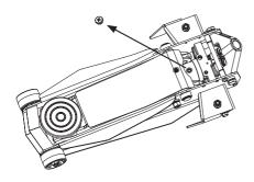
4. Fill the oil case until oil level is just beneath the lower rim of the oil fill hole.
