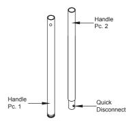
4. Unfasten the screw located in the Handle Socket to insert the assembled handle.
