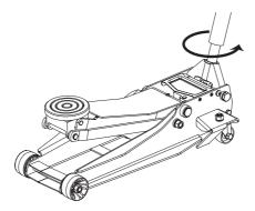
After removing jack from under the load, keep jack in the lowered position to reduce exposure to rust and contamination.
