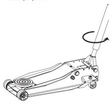
Rapidly pump the handle 6-8 times. Leave handle in down position to expose oil fill plug.
