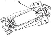
6.Replace coverplate and perform the Air Purge Procedure.
